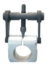
Lubrication: Use any quality oil on threads (not anti-seize) and any quality grease on load bearing surface in glove, under cap.
