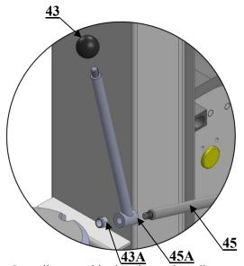
Install extend lock release handle and plastic ball
