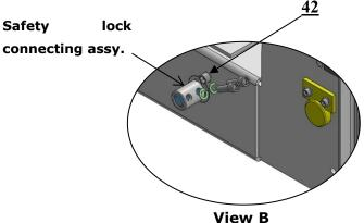
According to the above diagram, fix safety lock connecting bar and safety lock connecting by M8\*35 bolts and washers on cross beam B.
