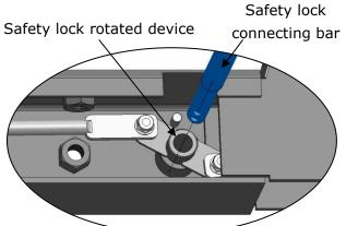
Pass through the connecting bar from the safety lock rotated device of cross beam **A/B**
