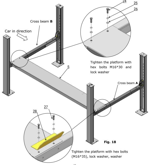
G.Install offside platform and plastic block, then install the bolts for the platform strengthen plate, check the plumbness of columns with level and adjusting with the shims (See Fig. 19)
