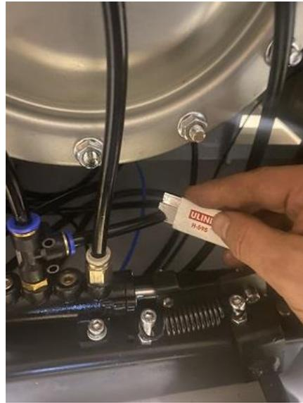
Connect the pneumatic valve that came from the assist arm in-between the two hoses that were spliced, as shown below.
