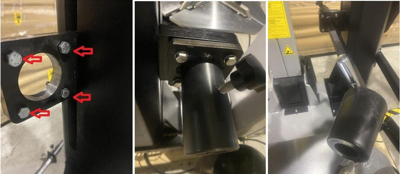
Pull out the pneumatic hose and valve that are rolled inside the assist arm's body. Disconnect the valve and route the hose through the hole in the side of the machine. Reconnect the valve inside the machine, as shown below.
