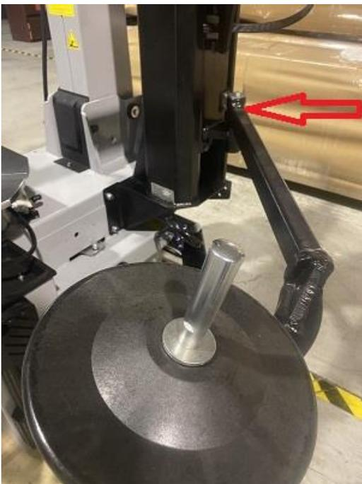
Loosen the four bolts from the square support attached to the tower of the assist arm
