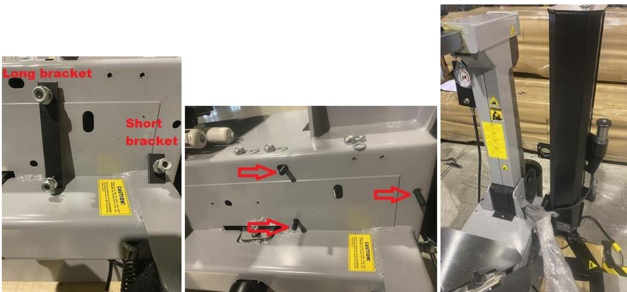
Mount the curved arm onto the arm that has the pneumatic lever, as shown below (Lubricate the areas that connect with white grease).
