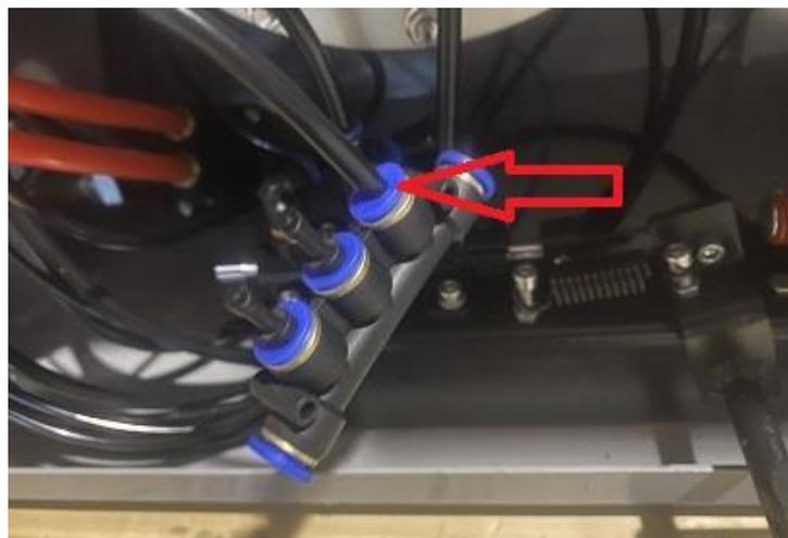
Splice the pneumatic hose coming out from the main valve assembly located inside the machine. Splice the hose approximately 3"-4" away from the valve, as marked with a red arrow below.
