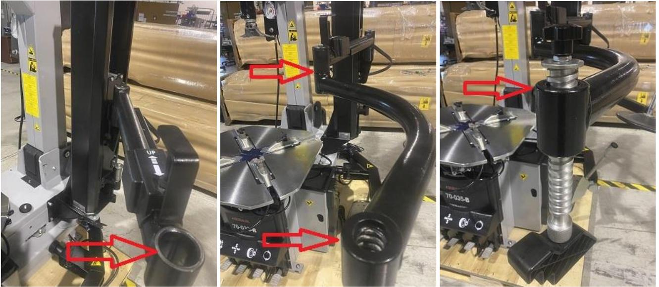
Mount the lower assist arm that has the rotating disc, as shown below. (Lubricate the areas that connect with white grease).
