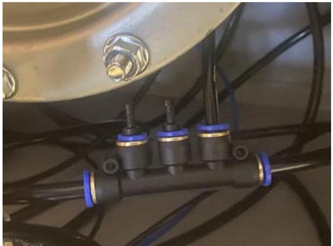
Re-mount the filter assembly in the back of the assist arm and re-connect the pneumatic hoses that were labeled in a previous step, as shown below.
