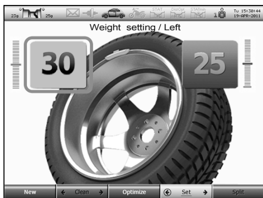
a - set the weight of 30 gr. on the left
