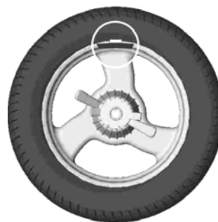
a - display image while clip-on weight setting b - weight is set in the position “12 h”
