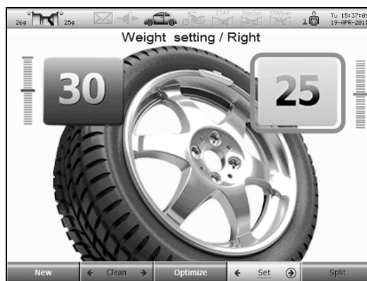
b - set the weight of 25 gr. on the right
