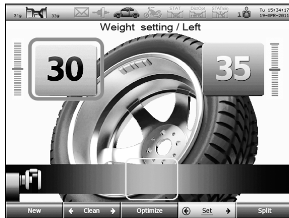
Figure 5.13 - Display image while the weight setting by the gauge arm
