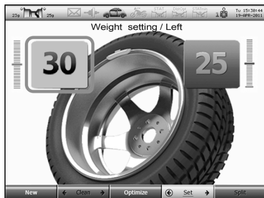
a - display image while clip-on weight setting b - weight is set in the position “12 h”
