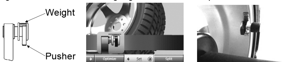
Figure 6.13 - Weight setting by gauge arm
