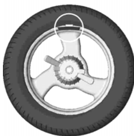
Figure 6.6 - The weight is set in the position "12 h"
