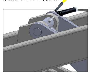
For shaft of piston rod of Main cylinder(1 moving parts)
