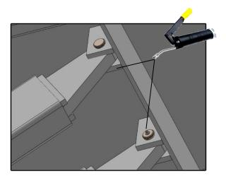
For pins of connecting platforms and scissors (2 moving parts)
