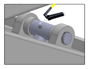
For shaft of piston rod of Secondly cylinder (1 moving parts) Fig.51
