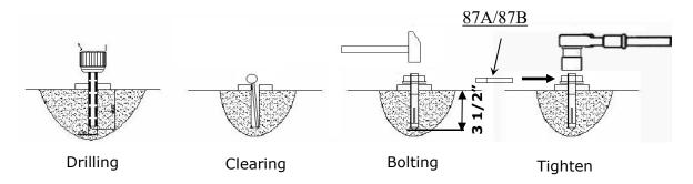
For the lifts: use  $\Phi 3/4$ " driller to drill hole For the control cabinet: use  $\Phi 3/8$ " driller to drill hole
