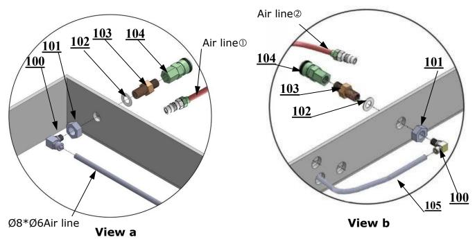
1.5 Install quick female fitting, then connect it with male air line  $\ensuremath{\mathbb{O}}$
