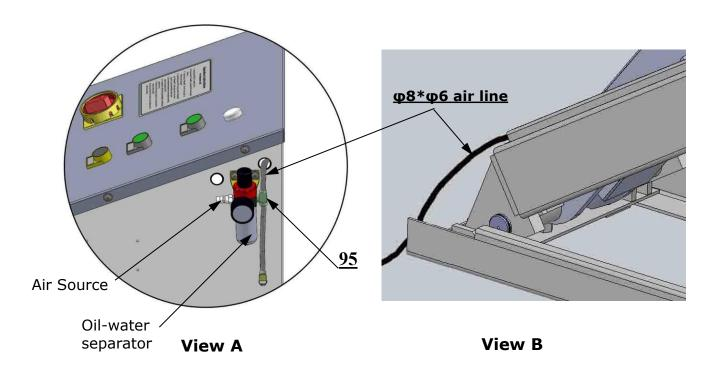
1.2 Replace 90° air hose fitting to three ways fitting from oil-water separator, then through black air hose( $\phi 8*\phi 6$ ) to control cabinet and connect with screw fitting.
