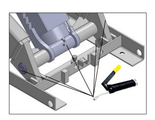
For Main Cylinder (5 moving parts)
