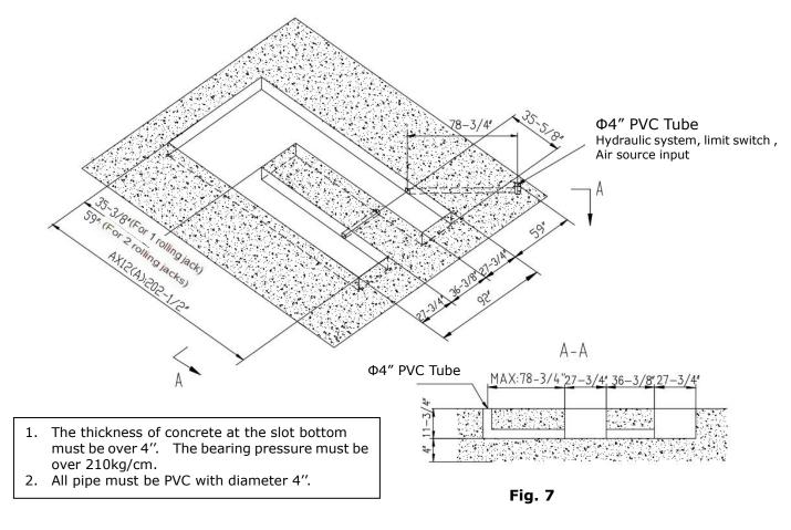
2.2 Illustration of scissors lift AX-12 with flush mount installation (Fig.8).
