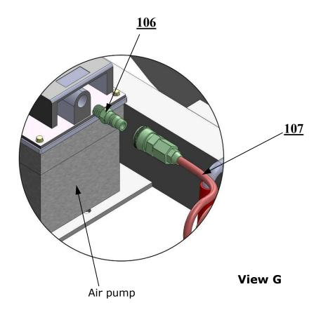
1.7 Connect female airlines of  $\ensuremath{\mathbb{O}}$  and  $\ensuremath{\mathbb{Q}}$  to quick male fitting on two operate jack
