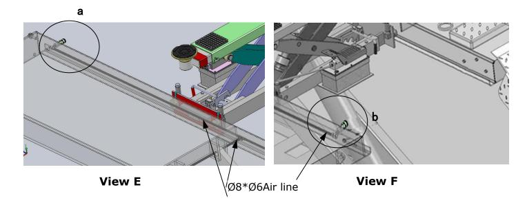
1.4 Air source divide into two ways by passing three ways fitting and connect with rolling jack separately.
