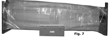
2. Move the lift aside with a fork lift or hoist, and open the outer packing carefully, take off the parts from upper and inside the column, take out the parts box, check the parts according to the shipment parts list (See Fig. 8).
