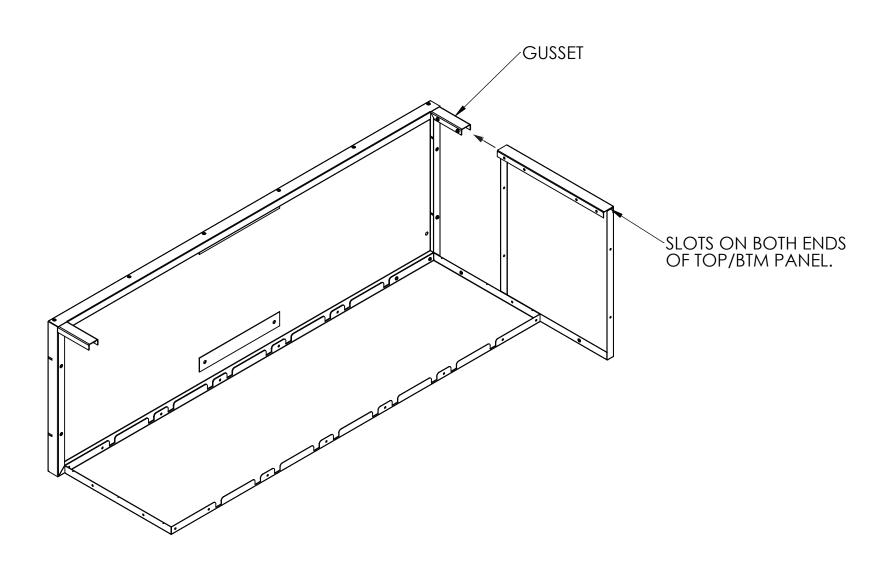
STEP 4: SECURE TOP/BOTTOM PANEL USING (4) M4 SCREWS
