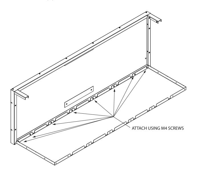
STEP 3: SLIDE A TOP/BOTTOM PANEL THROUGH ITS SLOT ON TO THE GUSSET OF THE SIDE PANEL.
