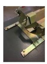
6. The side extensions can be mounted by inserting the square tube channel into the center table.
