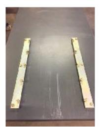
5. Mount the rails as shown. This will allow you to keep it on the table for motorcycles or loosen the bolts to remove it from the center table if not being used. Make sure to place the pins in the desired spot to fit your wheel accordingly, and if you have a narrow tire, the wedge can be installed to help secure the tire.
