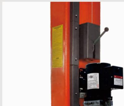
• Single point safety release makes it easier for operators to unlock both columns from one column.
