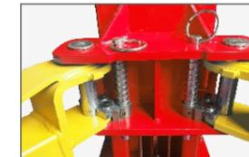
Lifting arm lock automatic release device, high strength gear rack, more stable and safer.
