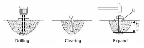
Note: Minimum embedment of anchors is 3-1/2"(90mm).
