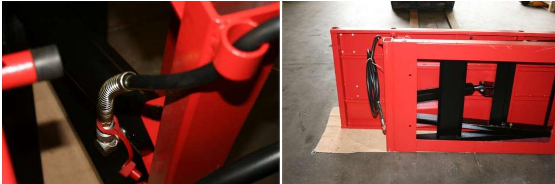
6. While one person steadies the lift, the other person slide the hydraulic hose through the guide (at the base of the lift) and connect to the hydraulic cylinder.
