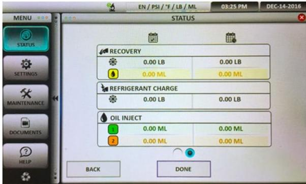
The values on the left side of the screen will display the last amount of recovered refrigerant, refrigerant charged and oil injected. The values on the right side of the screen display the lifetime totals of recovered refrigerant, refrigerant charged and oil injected.
