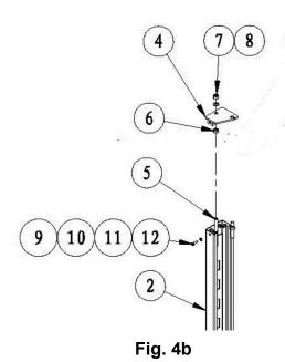
Secure Top Cap and Lock Ladder assemblies together with Washer and Nut as shown in Fig
