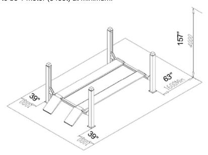
**OPERATING CONDITIONS:** Lift is not intended for outdoor use and has an operating ambient temperature range of 41°-104°F (5°-40°C).
