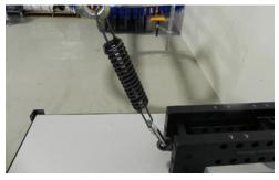
4 Attach the spring assembly to the eyebolt and the O/H crane.
