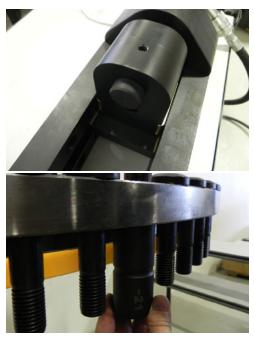
2 Attach the small button adapter (-18) to the cylinder end.
