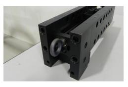
3 Remove the two small eyebolts and return them to the case. Attach the large eye bolt to the end of the tool.
