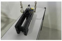
2 Attach the overhead crane to the eyebolts and carefully remove the tool from the box and place on a solid flat surface.
