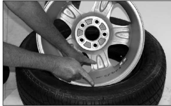
Figure 14 - Verify Size Match Between Tire and Wheel
