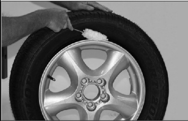
Figure 5 - Apply Rubber Lubricant to Tire Beads
