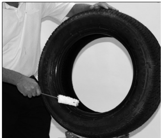
Figure 16 - Lubricate Tire Beads Liberally
