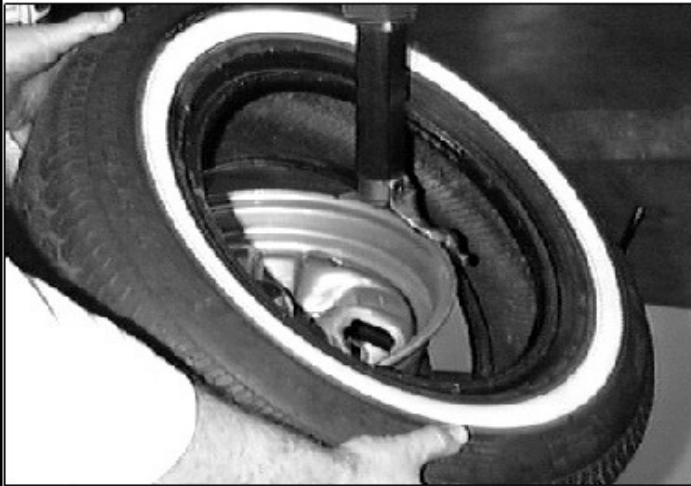
Figure 17 - Position Tire Against (Mount/Demount Tool)
