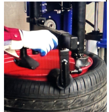
(Figure 9). Assist arm to help pressing the bead
