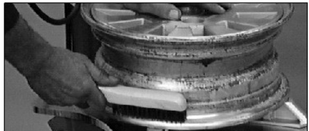
Figure 15 - Inspect and Clean the Wheel
