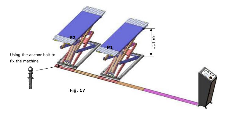
2.2 Drilling the hole for the anchor bolt with the rotary hammer drill, type the anchor bolt into the ground, and then fasten it with Ratchet spanner.
