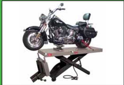
The S.A.M.2 Lift is designed to lift bikes up to 1000 lbs. This lift was developed for bike professionals who need a longer (93") and wider (28") work surface, with the convenience of double drop panels (15" x 28") for easy maintenance.
