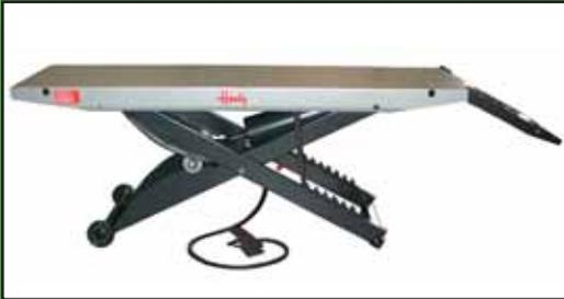
The Handy Air Lift has a lifting capacity of 1000 lbs. and an 80" x 24" deck, ideal for working on motorcycles, ATVs, snowmobiles, garden tractors, etc. It raises to a working height of 30" and lowers to 7" for easy loading. Solid steel fabrication and is powered by a pneumatic cylinder from your air source (90-100) psi. Can be used with or without accessories. W:24" x L:80". CE Approved.
